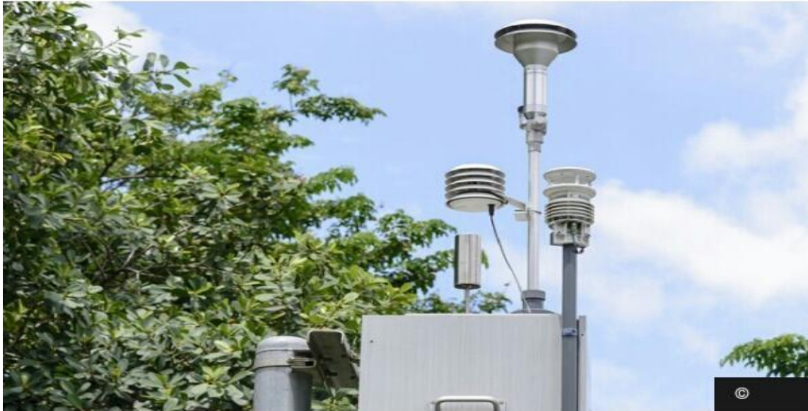
Fig.1: Picture of the routine GAIA Air Quality Monitoring Instrument with mounted sensors.
